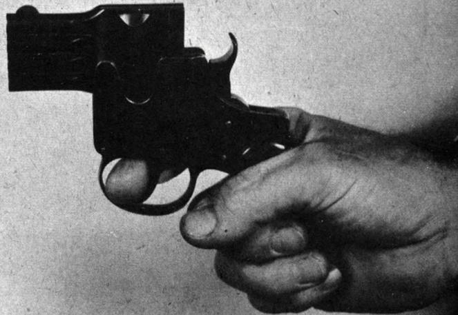
Here is a gun which has four barrels. After each shot whole barrel area rose to present new bullet.
